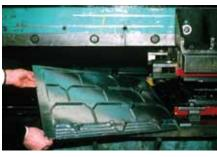
A surviving pressed metal shingle was used as a prototype for manufacturing replacement shingles when restoring the main house at the Motherwell Homestead near Abernathy, SK. In Restoration, repairs or replacements of extensively deteriorated or missing parts of features are done in kind, and are based on physical, documentary and oral evidence.
